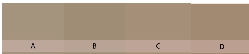
Fig.1: The leathers dyed with horse chestnut extracts (0.1 %NaOH; A 10; B 20; C 40; D 60g/L; suede side)
